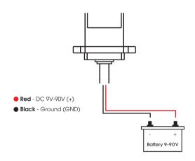
This tracker is designed for use on a vehicle. Testing the tracker on a separate battery or household battery household battery is not recommended. Place the tracker directly to the vehicle's on-board voltage or starter battery for which it is intended.
